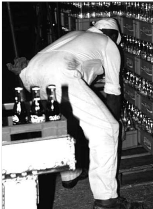
Figures 13 and 14 Examples of unnecessarily awkward working postures. Easy access to loads is critical to reducing strain. See Figure 37, p67.
