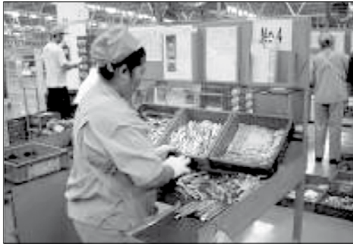
Improved access to materials using a tilt stand.
